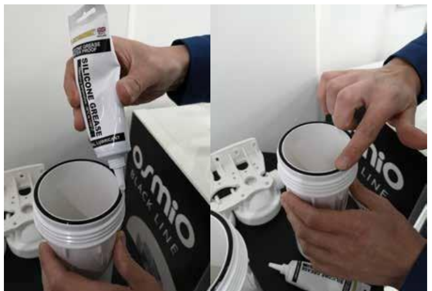
FIG4: GREASING THE O RINGS
